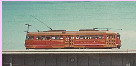
Figure 11- Actual Pacific Electric PCC car
